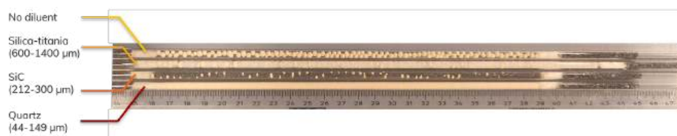
Figure 1. Image of a filled single-pellet-string quartz reactor to visualise the reactor loading of the spherical shaped catalysts.
